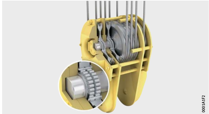
Figure 2 Rope sheave bearings in the example of a hook block
