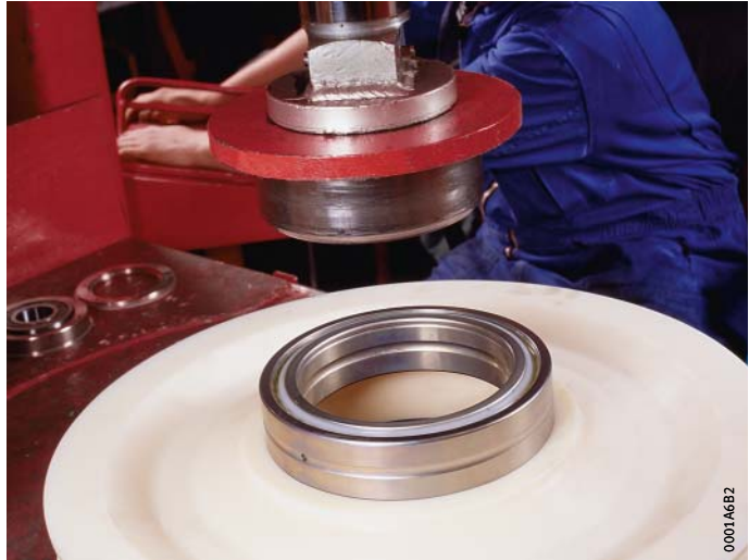
Figure 4 Mounting with control of force and travel
