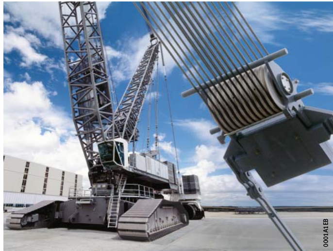
Figure 1 Rope sheaves in the Liebherr crawler crane
